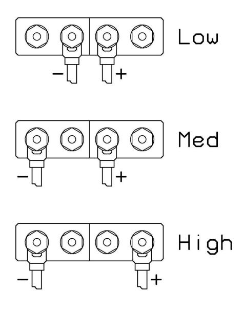
Figure 1 Output Connections
