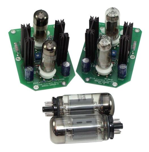
In its standard configuration the VK-80 current sources use the Russian 6C19 tubes. That tube is basically a miniature version of the famous 6C33 tube, and provides, in our view, the best combination of sonic characteristics and electrical performance.
